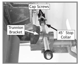
Figure 92. 45° stop collar and cap screws.
